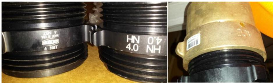
Figure 1. (INCORRECTLY SIZED FITTINGS - 4 THREADS PER INCH)
