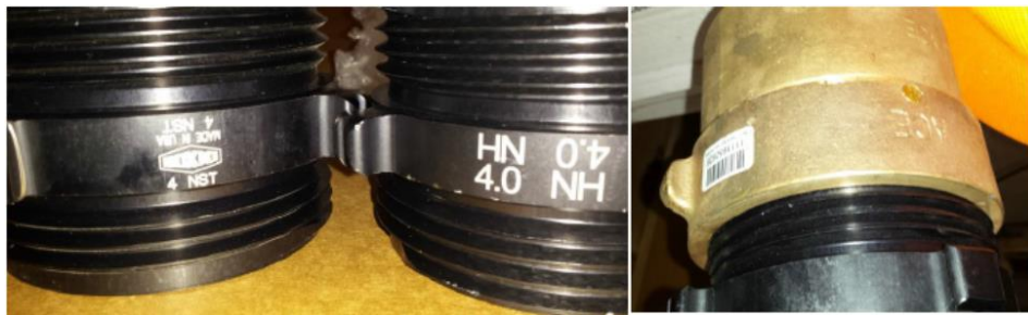
Figure 1. (Incorrectly sized fittings)
